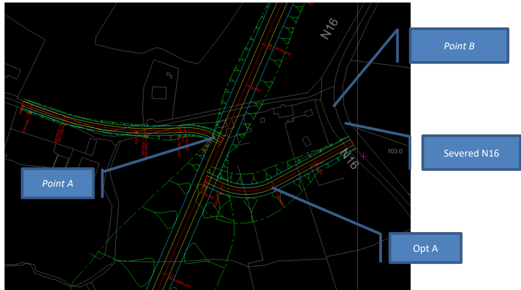
Figure 2-11: Option A: Simple T Junction at Lugatober (EAST) – Ch. 1,315m
