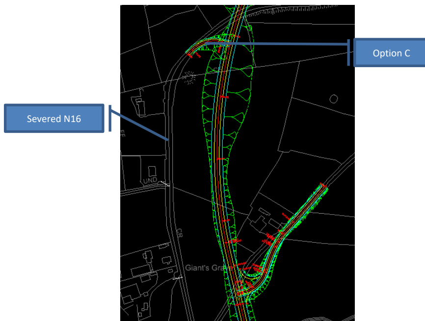
Figure 2-9: Option C: Simple T Junction direct connection at Lugatober
